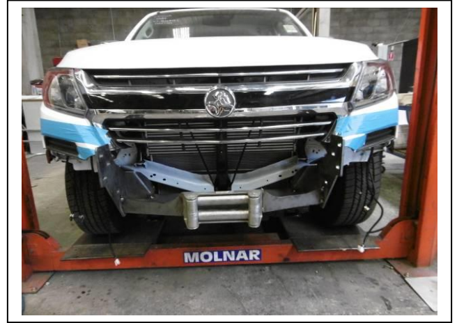
Figure 16: Cut across grille to fit over steel mount leaving grille mount on grille.
