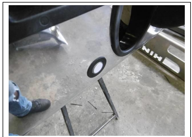
Figure 14: Sensor fitted into housing in protection bar.
