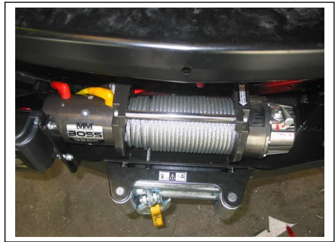
Figure 12: Install winch in winch frame as per manufacturer's instructions
