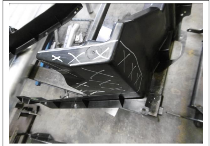
Figure 10: Trim line L/H air scoop
