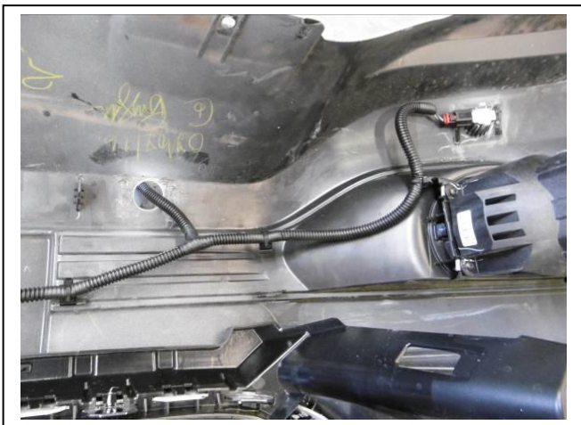
Figure 13: Remove sensors and wiring from bumper bar.
